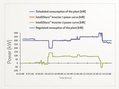
Our IntelliStore™ 1000 has been connected to a gas-fired electricity generator plant. With its 900 MW installed generator capacity the plant is an ideal site to use the storage device for ramping and phasing services. If idle, the plant's own electricity usage is optimized - no peak prices need to be paid.
