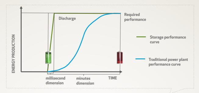
For ramping service our storage resources can help traditional energy producers e.g. gas turbines, to fulfill generation demand increases with steep gradient.
